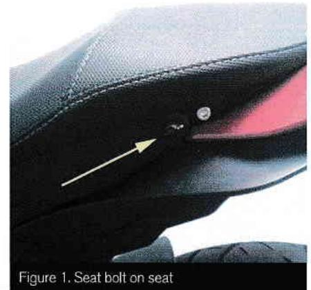
Figure 1. Seat bolt on seat
