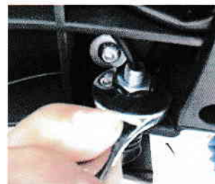
Figure 5. Remove turn signal hex nuts
