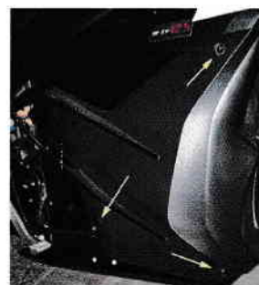
Figure 6. Remove battery fairings
