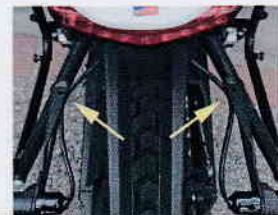
Figure 19. Signal wire secured to rear support
