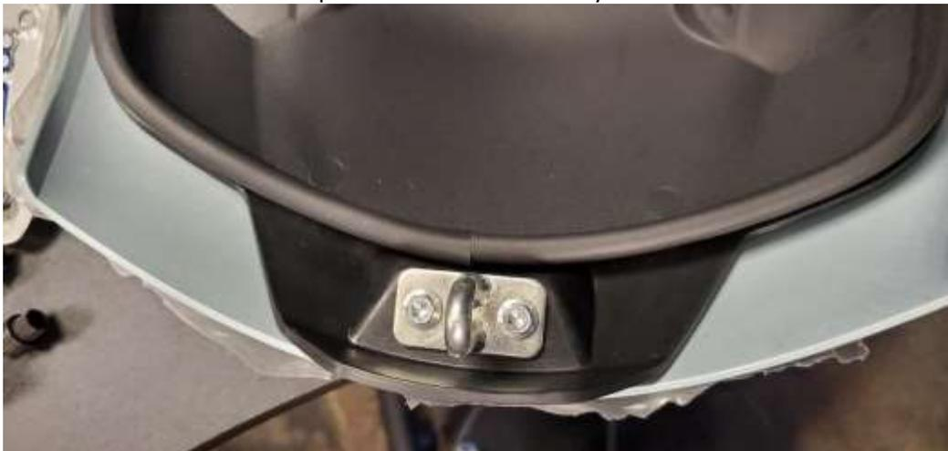
9. Install the Tank Trunk Latch Loop on the new Tank Trunk Lid Assembly using the M5x16 hex flange star drive bolts. Tighten to hand tight.
