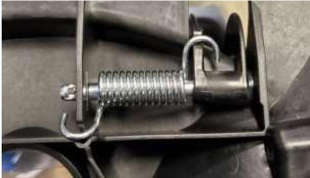
11. Reattach the Tank Arm Outer Left and then Right to the tank assembly using the #2 Phillips head screwdriver and the retained Phillips head screws. Tighten to hand tight and take care not to overtighten.
