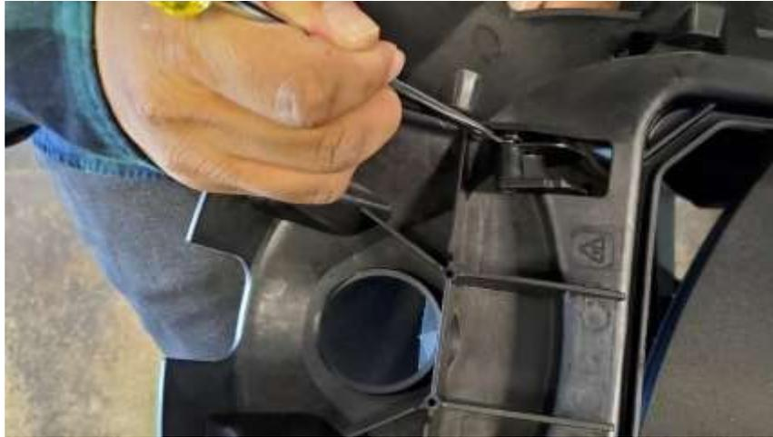
8. Using a TORX T25 screwdriver, detach Tank Trunk Latch Loop by unscrewing the M5x16 hex flange star drive bolts. Retain the latch loop and bolts for reassembly.
