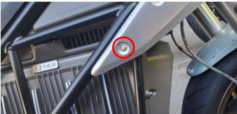
3. Using the #2 Philips head screwdriver, remove the seven Phillips head screws from the inside of the Tank Arm Outer Left to detach it from the tank assembly. Retain all parts for reassembly.
